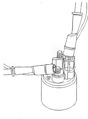
COMPONENT TESTING AND REPAIR Checking solenoid switch Use tester to check resistance of holding winding (term. 50/ground). Alternator tester: 0 684 201 200 Resistance for starting motors 0 001 124 0..: 1,5...1,7 Ohm 0 001 125 0..: 1,0...1,2 Ohm
